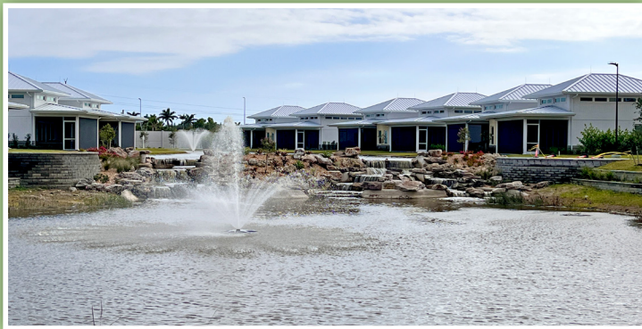
Two fountains and a cascading rock waterfall work together to enhance water circulation and promote healthy aeration, with water being pumped from the lower lake to the upper lined lake creating a visual and functional feature.
