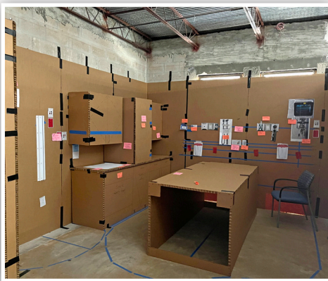
The cardboard setup allows clinicians to move doorways, walls, and equipment around to ensure both personnel and tools are optimally placed to provide the most efficient patient care possible.
