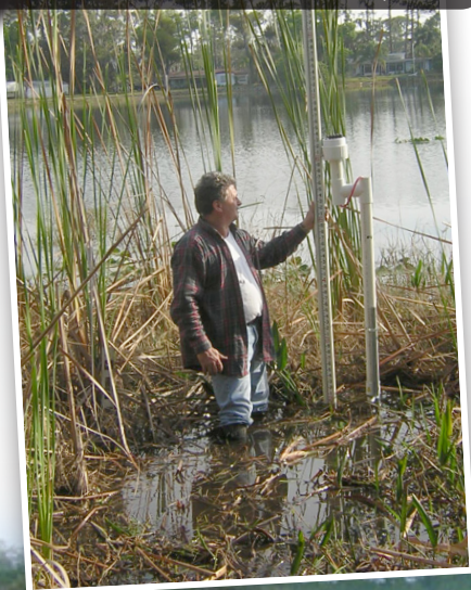
Mike checking setup for water level recorder at Lake Catherine in Seminole County.
