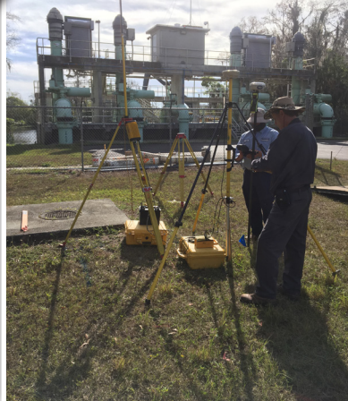
Survey crews used on-board GPS and hydrographic gear to map the depth and configuration of the river bottom.
