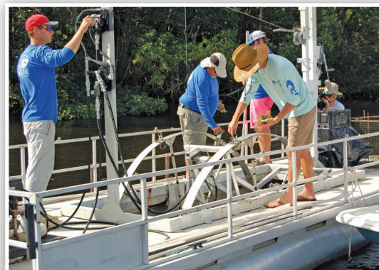
The team plants hundreds of seagrass pods using a mechanical planting barge with two large wheels that spin and bury the pods in the Caloosahatchee River bottom.
